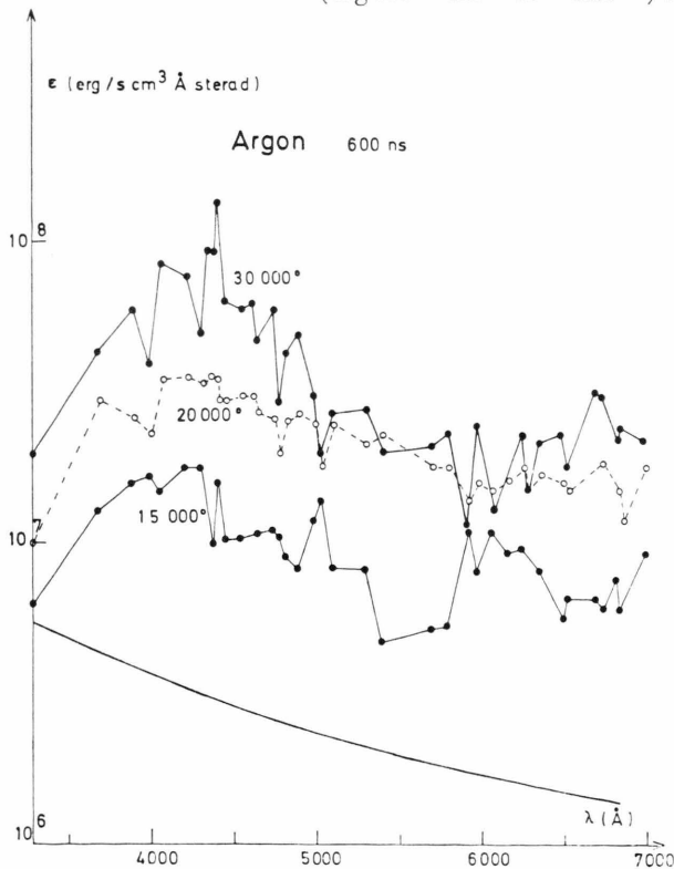
Fig. 1 a. The measured argon continuum at 600 nsec for different temperatures. The solid line shows the dependence of the emission coefficient calculated according to the Kramers-Unsöld theory. The pressure p is 3600 Torr.
